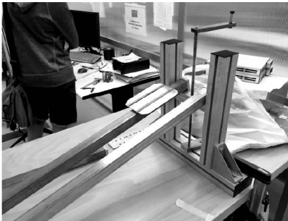
Figure 3. Smartphone based experience to measure friction coefficients of different materials
